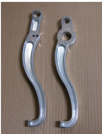
Figure 1. Here's the prototype pedals still sitting on my shelf, waiting to be completed. Note that the clutch replicates the OEM configuration, whereas the brake was designed as a dual master cylinder design with a balance bar which is not shown.
