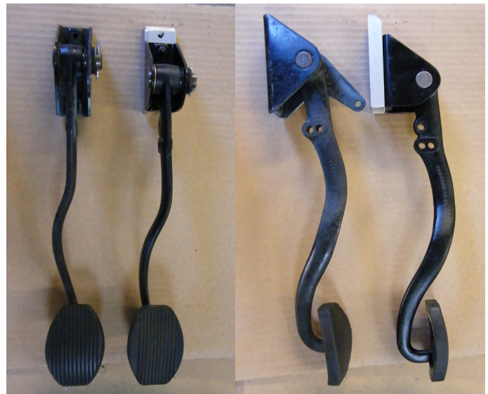
Figures 2 & 3. Here's a comparison of the OEM pedal and the MTE 6 to 1 modified brake pedal. The aluminum adapter that relocates the modified pedal pivot both back and down is shown. Also shown here is the relocation of the pedal pad, so that the pad remains the same distance from the floor.
