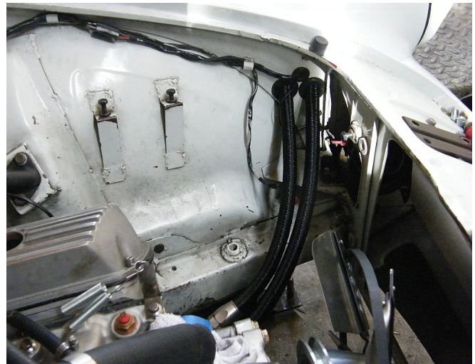
Figure 3 Here's the general hose routing to the side of the engine compartment. All neat and out of the way.
