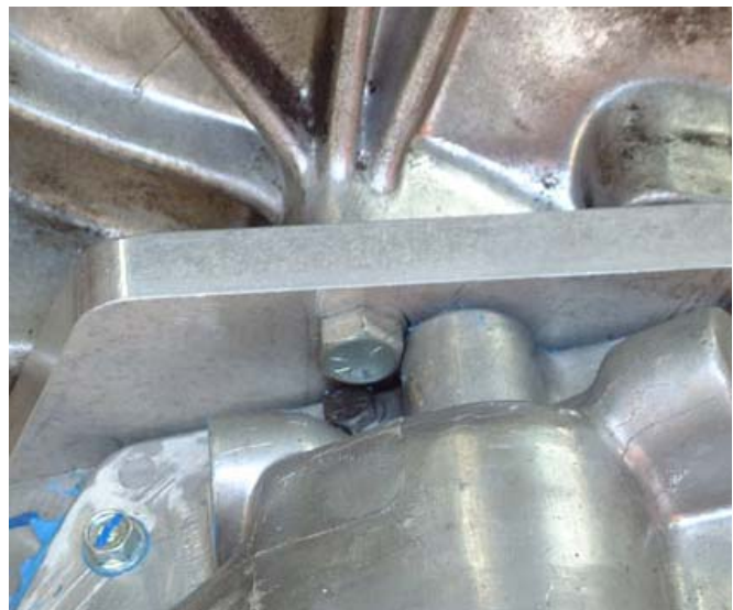
Fig 2 Turn the hex on the five bolt adapter as shown.
