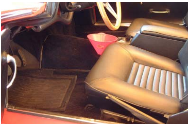
Fig 10 Here's the funnel I use to add the required Lubricant BEFORE installing the shifter mechanism.
