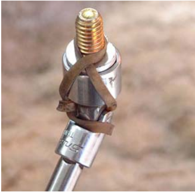
Fig 12 Here's my trick for holding the screw and lock washer in the socket while you position it, screw down, through the RTV into the shifter and tailhousing.
