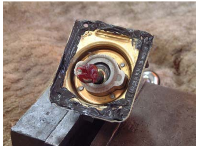
Fig 11. Here's the Modified T56 shifter ready to drop through the stock shifter hole into the tailhousing. A blob of grease lubricates the ball where it slips into the nylon bushing.
