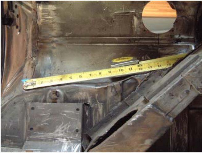
Fig 8 Another chassis, same alteration. This dent is the area where the bolt was removed from the side if the T5 transmission. If you made this dent another inch deep, the transmission would fit without removing the bolt.
