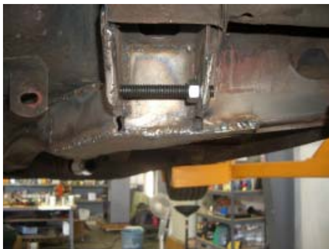
Figure 14. Here's my drill fixture. It's a piece of 7/16 threaded stock with a 1/4" hole drilled through the center. Inserting this piece and tightening the nut as shown, allows the center of the inner hole to be pilot drilled avoiding any enlargement of the original 7/16 hole.
