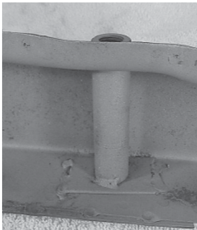
Figure 15. This is what you'd find if you looked inside the front frame horns. As you can see, the tubenut is simply tacked in place.
