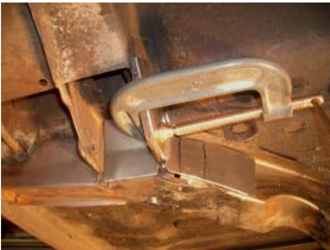
Figure 10. Here's the side piece and the front piece clamped into position, ready for tack welding.
