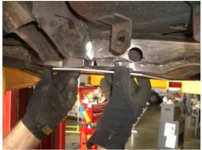
Figure 12. The bottom plate should be a pretty close fit to the side and inside piece where they will be welded together. Some angular adjustment may be necessary with the sanding belt. It's also a good idea to hammer the metal to form joints that can be welded into a tight configuration so that the end result is as smooth and uniform as possible.
