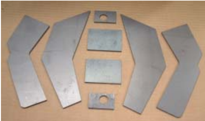
Figure 1. Here are the pieces that make up the MTE Reinforcement Kit. They include three plates for the rear spring mount area for both sides and the plates for the front Tubenuts at the front crossmember.
