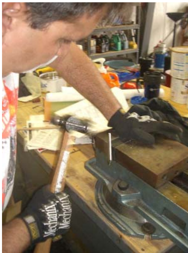
Figure 7. Here you can see how the side plate is bent to fit. Take your time and work this piece gradually. It's easier to bend it a little at a time than to unbend and rebend. If the location of the bend is not obvious to you, cut a replica out of cardboard and fit that first. Then transfer the bend location to the steel piece.
