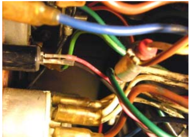
Figure 8. This photo shows the Red LED inserted into the rear of the red warning light housing.
