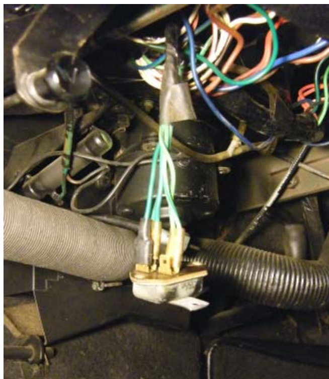
Figure 4. Here's the OEM Regulator pulled down for easy access.
