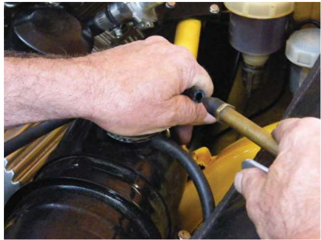
Figure 3. This is the method I use to vent the right hand radiator tank. You'll want very low pressure from your air system. Holding your hand over the Reservoir top fitting, allows you to apply a small air pressure, through the overflow tube, to the reservoir to force the coolant into the right tank until it flows out the vent tube. This completes the purging of air out of the coolant system.
