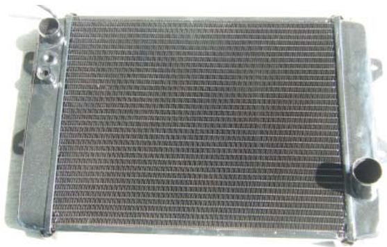
Figure 1. This radiator re-core uses your OEM tanks and sheet metal supports. The core is 2" thick, the same as the original core, but much higher efficiency. If your core has the top and bottom sheet metal supports flattened for a fatter core, they will have to be returned to the OEM configuration at extra cost.
