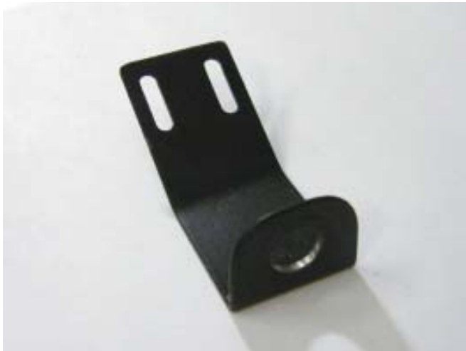
Figure 1. Here's the bracket that fits behind the brake pedal.
