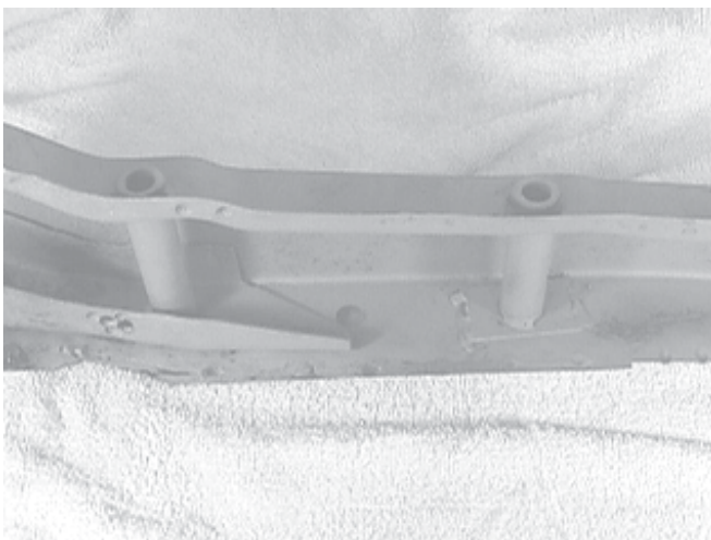
Figure 3. This shows both front and rear tubenuts and the stamped frame reinforcement inside the frame in the area of the hump and motor mounts. The plug welds you see on the side in the area of the rise connect to this internal stamped member. (Too bad the designers didn't bring this piece forward to the front tubenut!)
